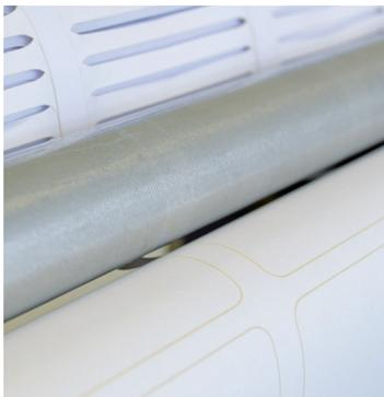
*The peeling rollers module facilitate the matrix removal from the die-cut roll, reducing the risk of tearing and ensuring more precise operation of the machine.*
