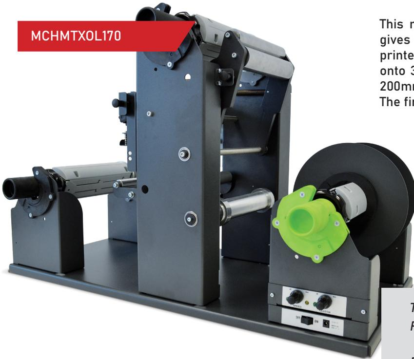
This new offline matrix remover version for Oki Pro Series gives the user the ability to remove the waste material from printed or blank pre die-cut rolls of labels up to 170mm wide onto 3" cardboard core and having an outside diameter up to 200mm.
